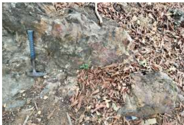
Field Photograph 7: Gossan zone within dolomite is the prominent indication of sulphide mineralization
