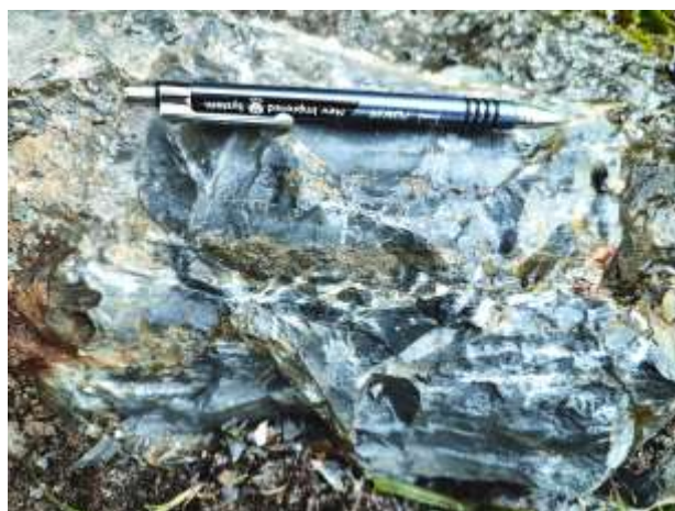
Field Photograph 6: Mineralised veins contains chalcopyrite, pyrite, galena within sheared dolomite
